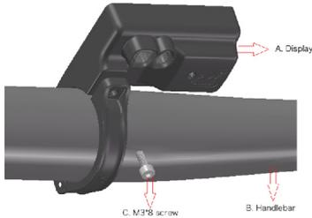
**i** Note: The diameter of display clamp is  $\Phi 35\text{mm}$ . According to the diameter of the handlebar you can choose whether to need a rubber ring ( $\Phi 22.2$ ,  $\Phi 25.4$  or  $\Phi 31.8$ ).
